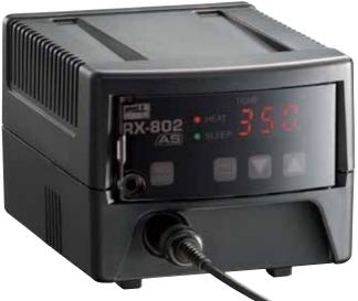
\*The station unit for the **XST-80** is our Lead-Free Soldering Station **RX-802AS**
