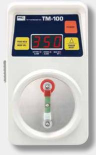
Wide temperature range \*0-700°C (1292°F), as is necessary for soldering work. The tolerance stays in the range of  $\pm 0.5\%$  of the full scale (excluding sensor error). The sensor's structure makes for easy tip placing. It achieves stable & accurate measuring within seconds, regardless of shape, or angle of tip. Easily replaceable sensor.
