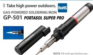
•Heats quickly. Takes only 30 seconds from ignition until soldering. Controls equivalent power of 25-125 W with the temperature adjuster. •Can be used as a blow torch by removing the tip. With optional tips, do soldering work for large metal or precision PCBs, or use as a hot knife or a hot air tool. Operates approx. 45 minutes between refills (when used at max. temperature as a soldering iron). •One-handed, one-touch ignition switch.
